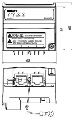
Please consider when attempting to install the WJ200 series that by attaching any of the WJ-ECT, WJ-PB or WJ-PN option, the inverter D (depth) size will increase by 26.3 mm regardless of the inverter capacity.
