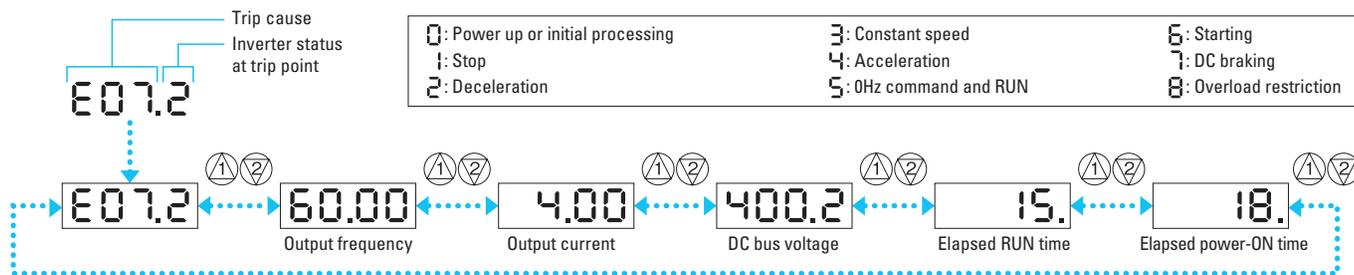
Note: Indicated inverter status could be different from actual inverter behavior. (e.g. When PID operation or frequency given by analog signal, although it seems constant speed, acceleration and deceleration could be repeated in very short cycle.)
