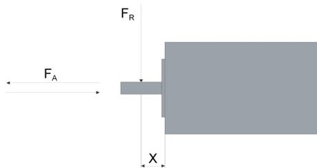
The point of application of the forces depends on the motor size:
