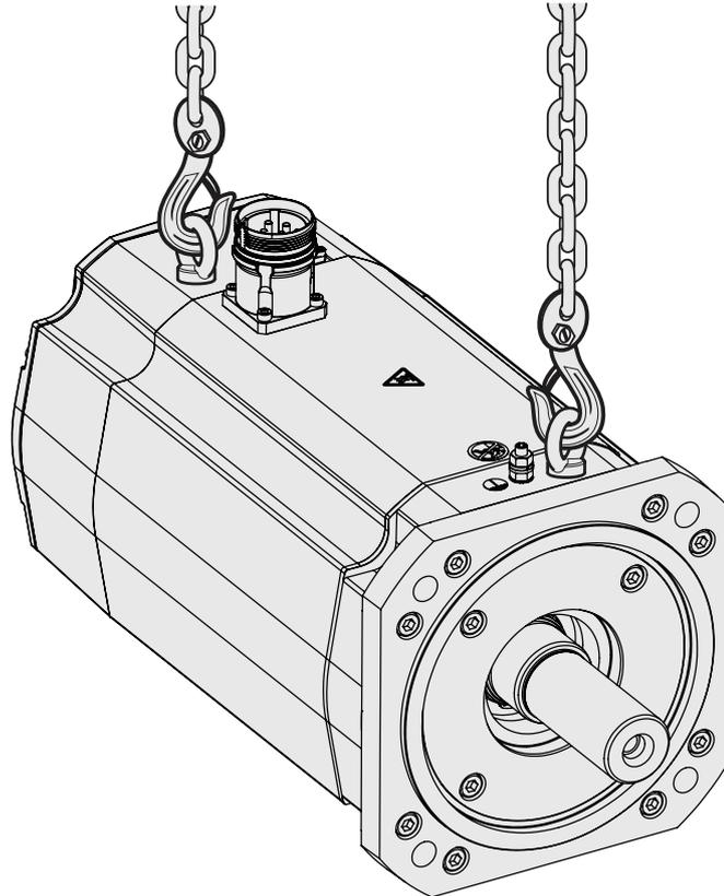
After the motor is mounted the eyebolts can be kept or removed. Remove the eyebolts if necessary, for example for rotating the connector.
