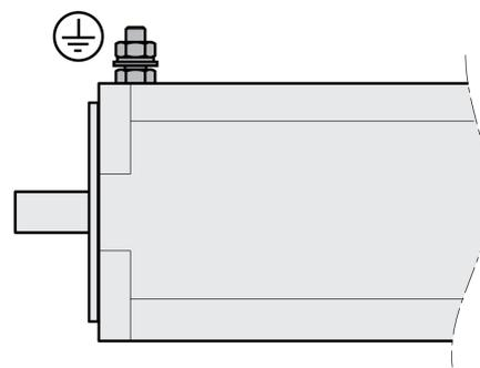
Ground the motor via a grounding screw if grounding via the flange and the protective ground conductor of the motor cable is not sufficient. Use parts with suitable corrosion protection. Note the required tightening torque and the property class of the grounding screw, see Tightening Torque and Property Class Of Screws Used, page 17.
