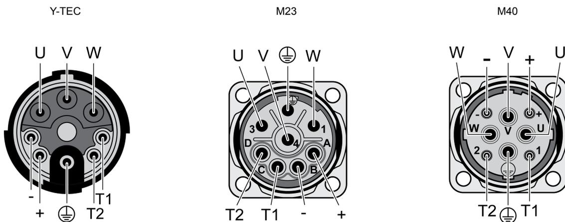
The circuits of the holding brake and the temperature sensor meet the PELV requirements.
