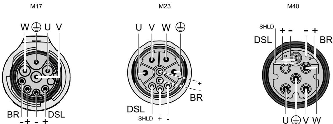
The circuits of the holding brake and the encoder meet the PELV requirements.
