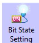
The Bit State Setting defines a touch area. When this area is active, this button can set the HMI bit address or PLC bit address On or Off. The display status of this component will not be changed by the input value.
