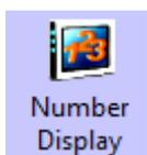
Number Display is used to display the value in specific HMI or PLC register on HMI.
