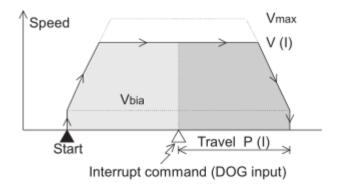
When the start command is received, the motor starts operation. When the INTERRUPT input is received, the motor moves by the specified distance, then stops (The relative travel exclusively can be specified.) The current value is cleared by the start command. The current value starts to change
