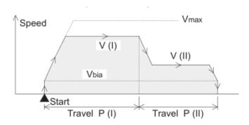
The motor performs the following operation by the two-speed positioning operation command. Approach at high speed as well as processing and moving forward at low speed can be performed. When the start command is received, the motor performs positioning at the operating speed V(I) (BFMs #20 and #19) until the set position P(I) (BFMs #18 and #17), then at the operating speed V(II) (BFMs #24 and #23) until the set position P(II) (BFMs #22 and #21) (two-step speed).
