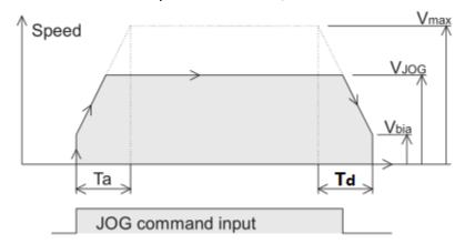
Any value between the bias speed  $V_{bia}$  (BFM #6) and the maximum speed  $V_{max}$  (BFMs #5 and #4) is valid as the command speed  $V_{JOG}$  (BFMs #8 and #7). When JOG signal continues to be 1 for less than
