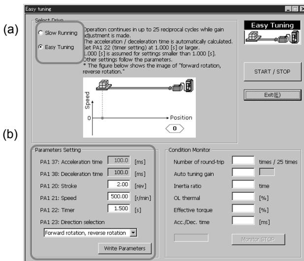
Press the "START/STOP" button to start one of motions (a). Press the START/STOP button during the motion to stop immediately.
