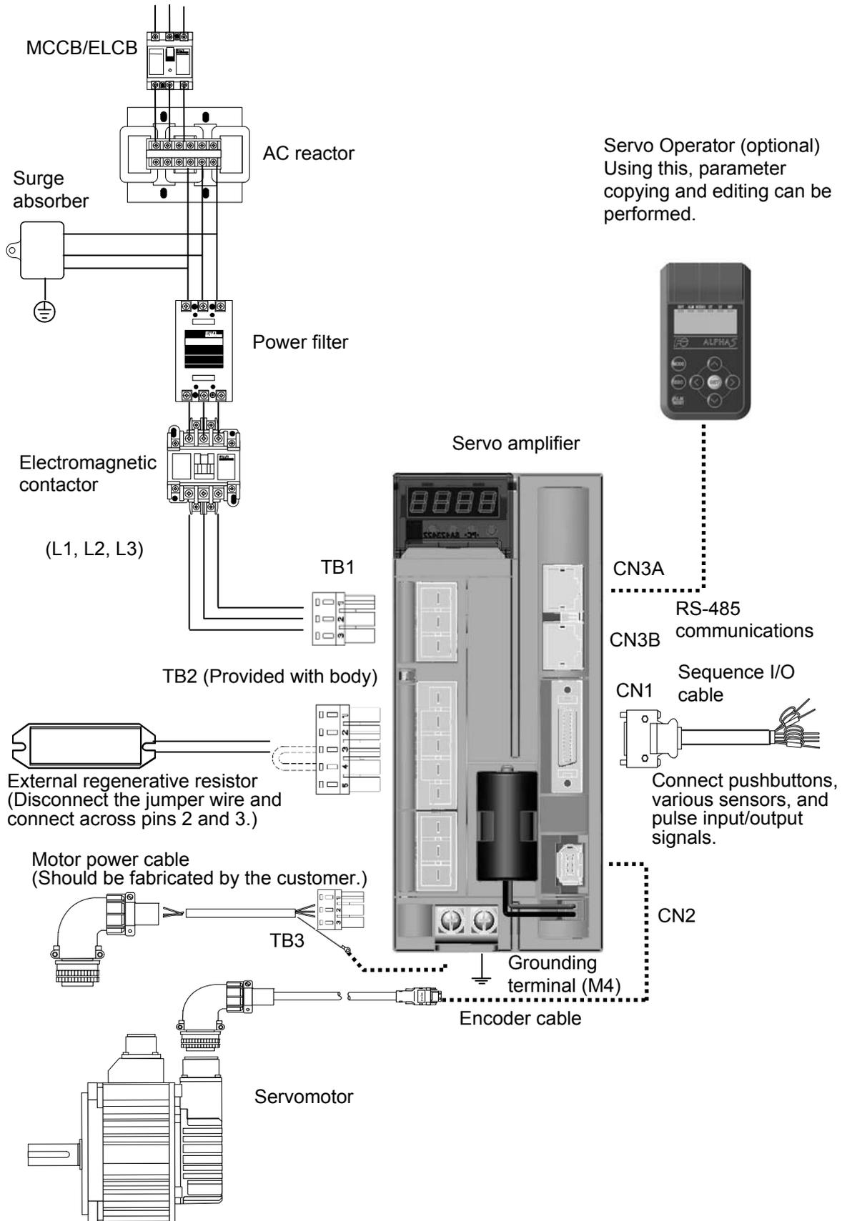
Sample Connection Diagram (Servo amplifier frames 2, 3 and 4)
