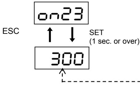
The servomotor power (w) is displayed in percent to the rating.
