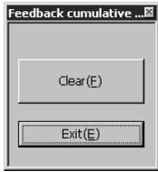
Press the "Clear" button to reset the cumulative feedback pulse to "zero."
