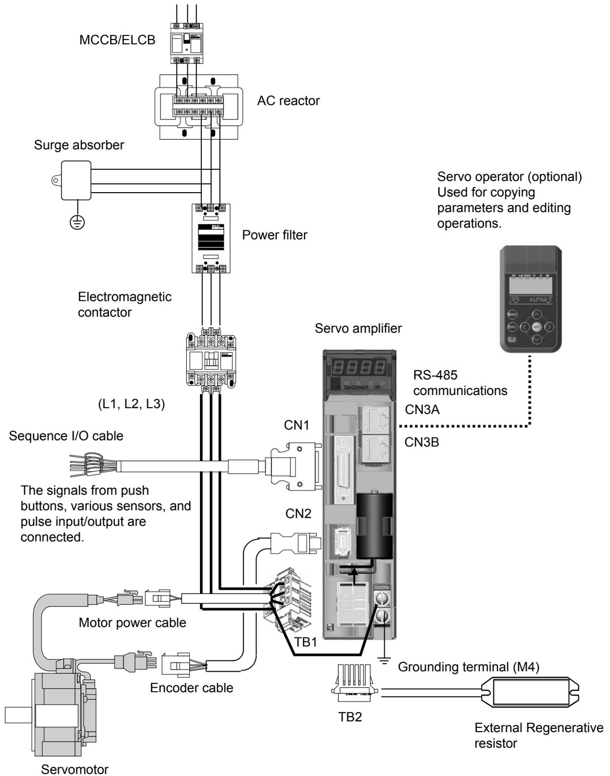
Sample Connection Diagram (Servo amplifier frame 1)
