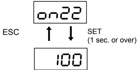
The regeneration load ratio to the regenerative resistor overheat alarm level is displayed in percent. A regenerative resistor overheat alarm is caused if this value is 100. The regeneration load ratio is calculated for amplifier frame no.2 or above if PA2\_65 (regenerative resistor selection) is set at 1 (internal resistor).
