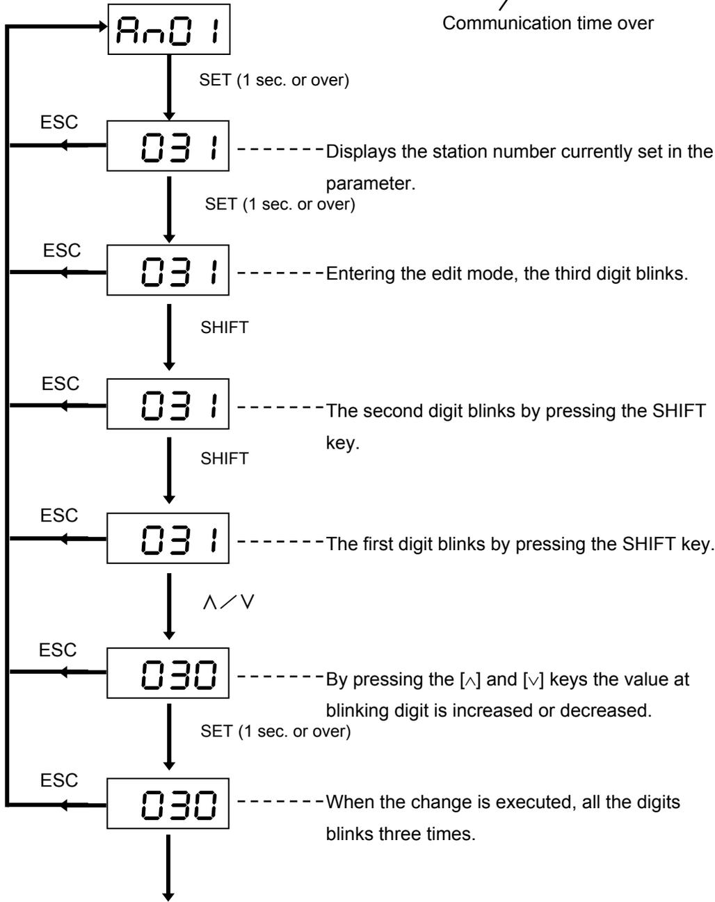
Turn the power off and on again to enable the new station number.
