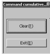
Press the "Clear" button to reset the command cumulative pulse to "zero."
