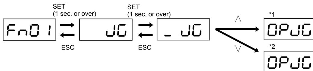
\*1) [During forward rotation ((^) being pressed)]    \*2) [During reverse rotation ((v) being pressed)]
