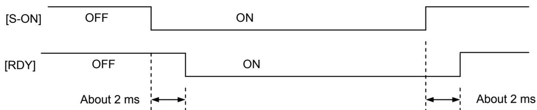
The servo amplifier input signal can be always enabled with parameters PA3\_26 to PA3\_30. Servo-on [S-ON] turned on before power-on does not cause breakage to the servo amplifier.
