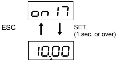
The input voltage of the analog input terminal [VREF] is displayed in 0.01 V. The negative sign indicates a negative voltage.
