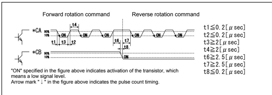
■ Differential input, forward/reverse pulse (reference value of parameter 03: 1)
