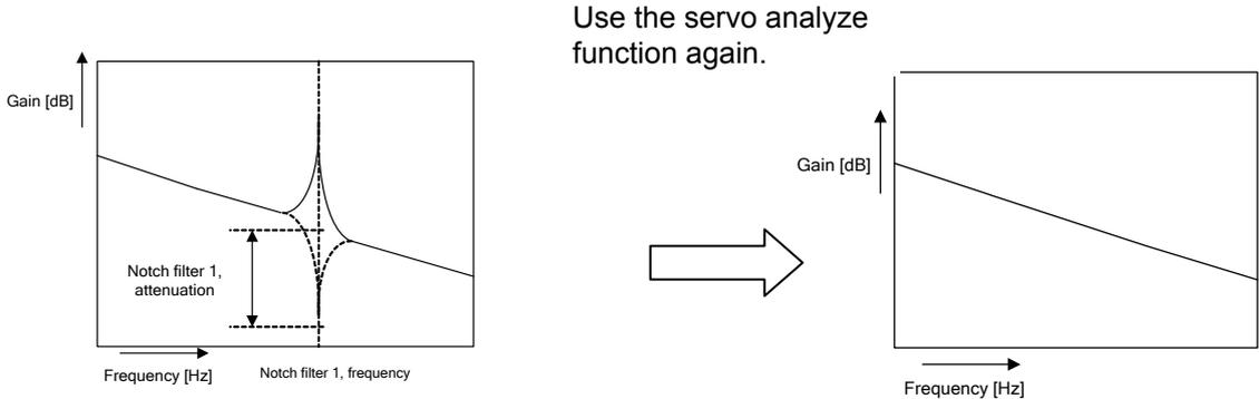
The notch filter is added to the resonance point as shown in the figure above.
