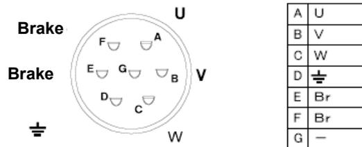
Recommended connector kit (motor side) for GYH type brake wiring
