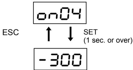
Current flowing through the servomotor; the current is displayed in percent to the rated current. The range from 0% to the maximum current is displayed in increments of 1. In case of a negative motor current, a negative sign is attached to the most significant digit.
