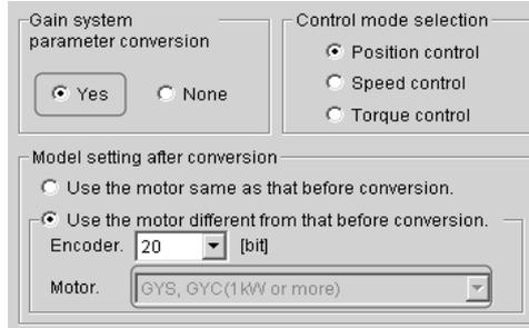
When “None” is selected at gain system parameter conversion, the motor model after conversion can be selected.
