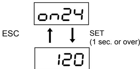
The servomotor temperature is displayed. The range from 0 to 120°C is displayed in increments of 1°C.
