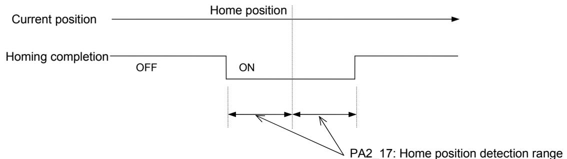
The home position is the stopping point after a homing motion is finished, or a position at which position preset is executed. It does not mean the "0" position.
