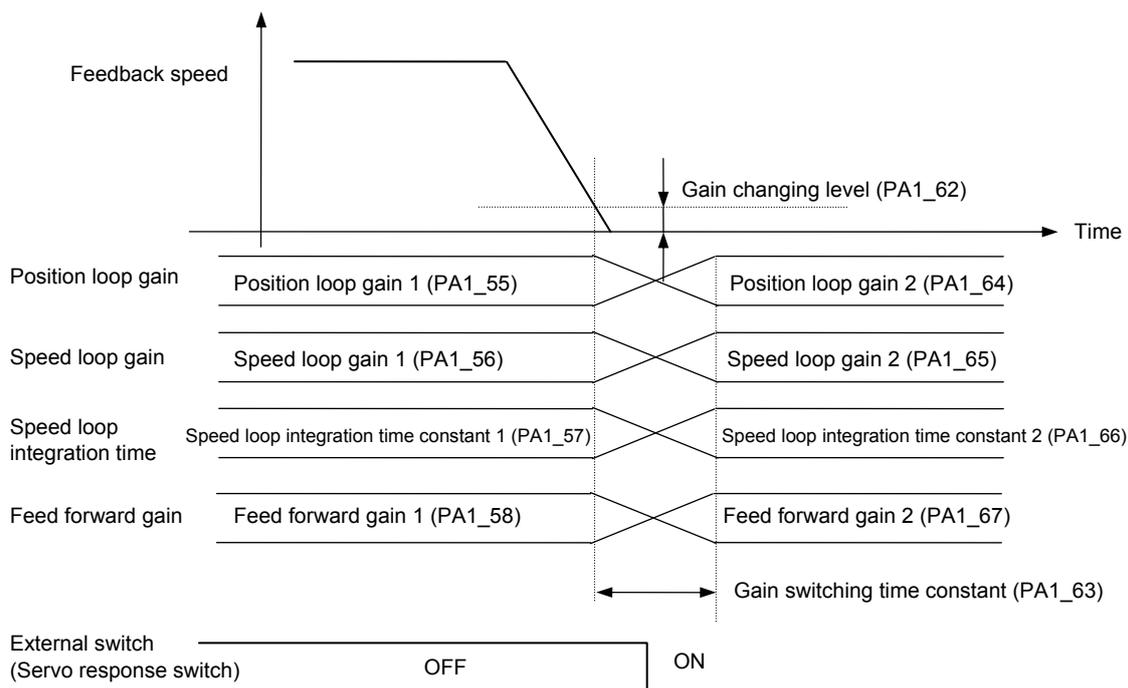
If external switch is selected as a gain changing factor, changeover to the second gain occurs during OFF-to-ON transition as shown above. In this case, you can turn on or off at an arbitrary timing without relations to the motor motion.
