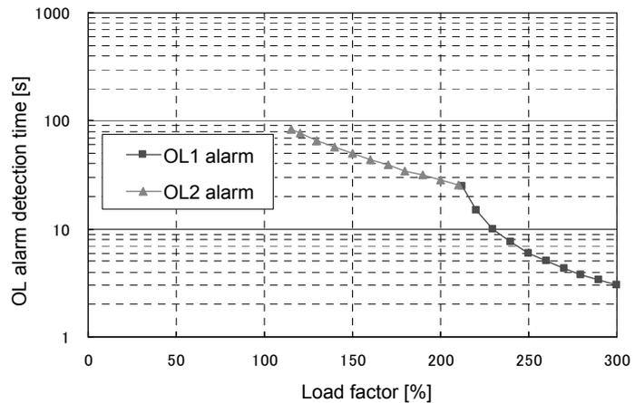
Note) The OL1 alarm detection time is 15 [r/min] or more. The alarm time will be detected in shorter time (0.25sec/300%) if the motor is stopped due to machine entanglement or other reasons resulting in overload.
