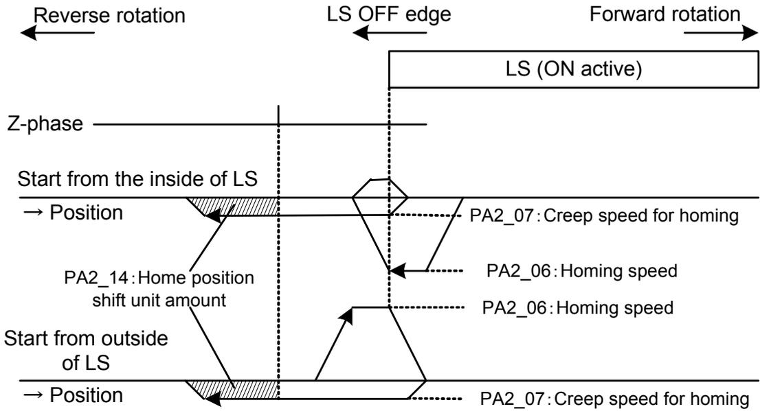
(7) Homing pattern using the encoder Z-phase as a reference signal for homing
