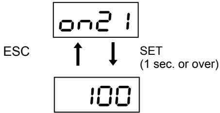
The load ratio to the load alarm level is displayed in percent. An overload alarm is caused if this value reaches 100. The minimum increment is 1. The displaying range is from 0 to 100%.
