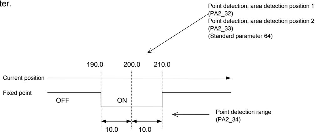
(2) Area OFF → ON (If PA2\_31 (point detection, area detection) is 1)
