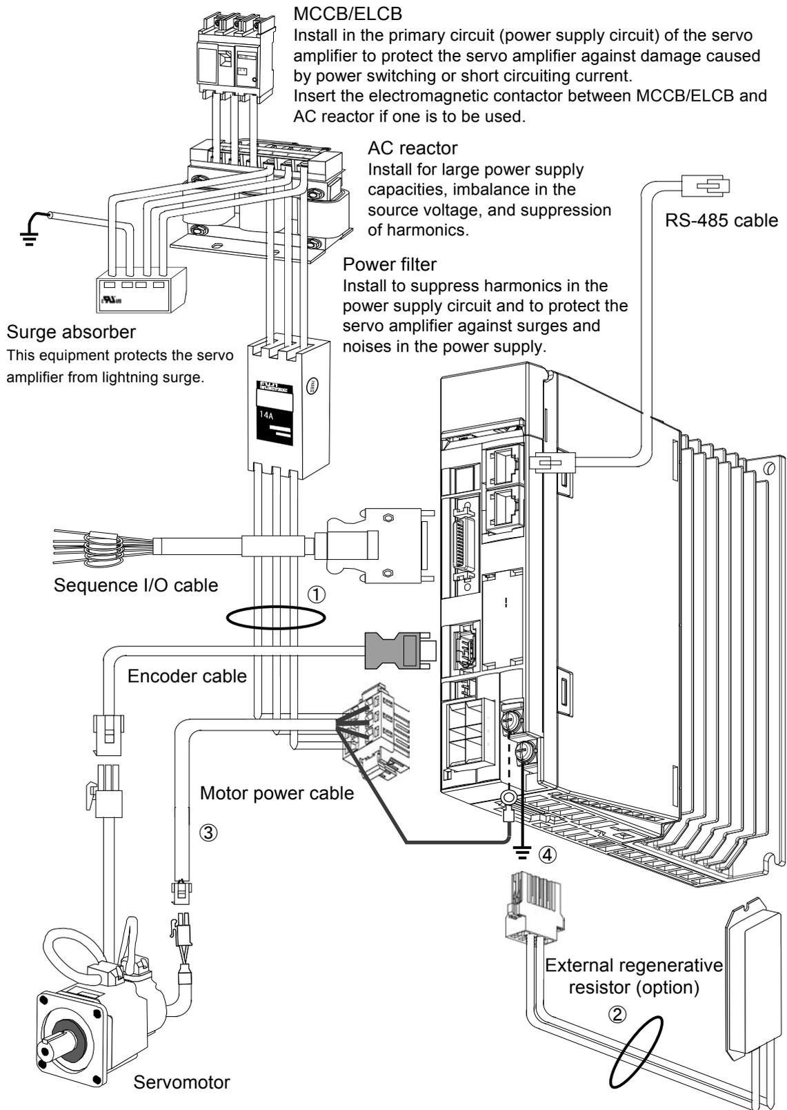
Wiring connectors do not come with the servo amplifier or servomotor. Prepare the necessary option cable or connector kit.
