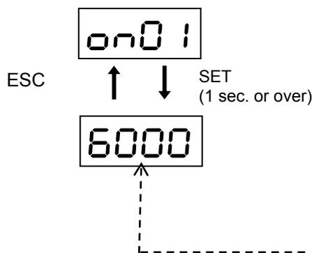
Current rotation speed of servomotor.
