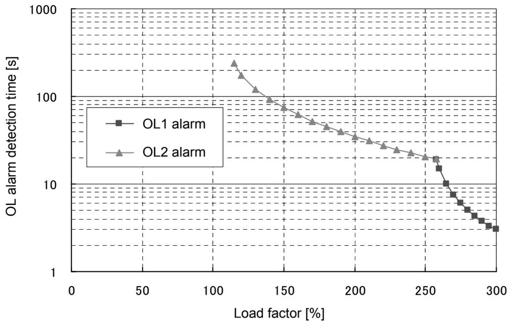
(2) In case of operation at maximum rotation speed (6000 r/min)
