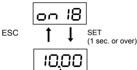
The input voltage of the analog input terminal [TREF] is displayed in 0.01 V. The negative sign indicates a negative voltage.
