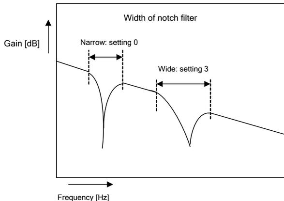
The notch filter is added to eliminate the resonance point.
