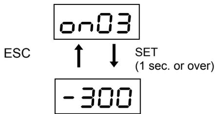
Average torque issued from the servo amplifier to the servomotor; the torque is displayed in percent to the rated torque. The range from 0% to the maximum torque is displayed in increments of 1. In case of a negative average torque, a negative sign is attached to the most significant digit.
