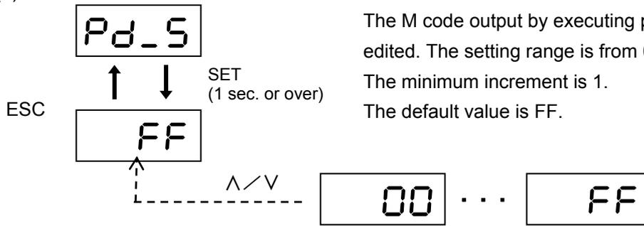
The M code output by executing positioning data can be edited. The setting range is from 00 to FF in hexadecimal. The minimum increment is 1. The default value is FF.
