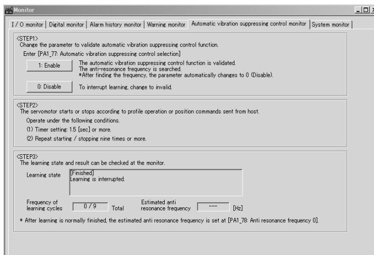
If no expected effect is obtained under automatic vibration suppression, refer to the following "5.10.3 Manual Adjustment of Vibration Suppression."
