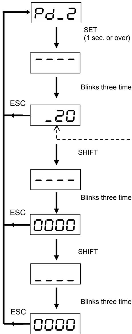
Set the target position of the motor. The setting value range is from -2000000000 to 2000000000 in increments of 1.
