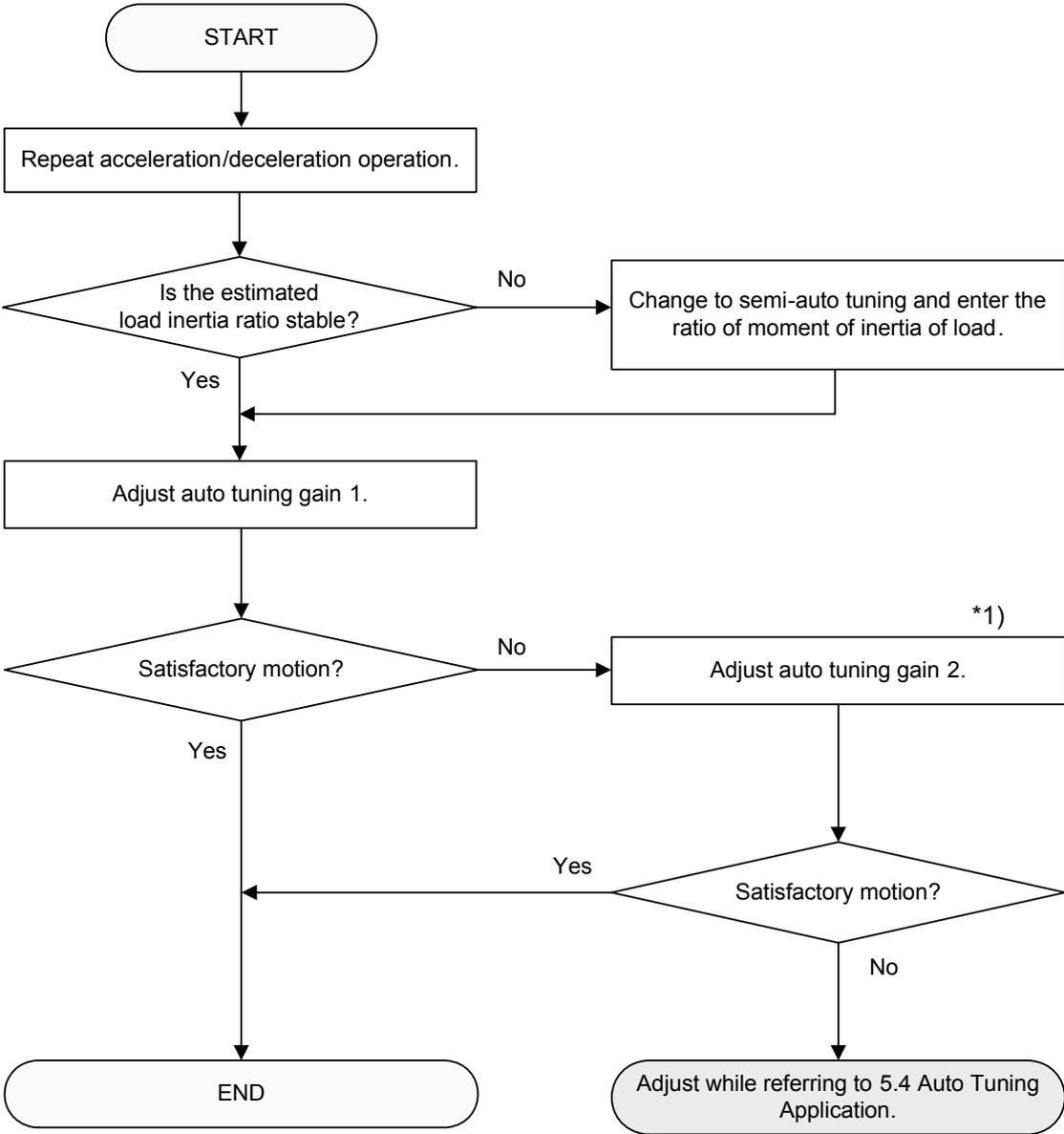
\*1) There is no need to adjust auto tuning gain 2 under speed control.
