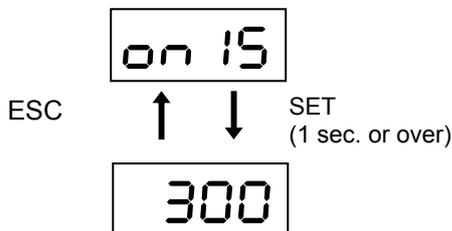
The DC link voltage (max.) of the servo amplifier at every two seconds is displayed. The displaying range is from 0 to 500 V.
