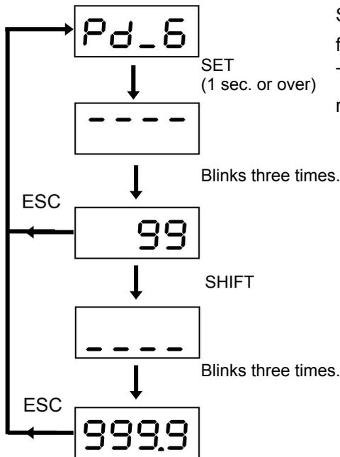
Set the motor acceleration time. The setting value range is from 0.0 to 99999.9 ms in increments of 0.1. The setting value is the time until the motor rotation speed reaches 2000 r/min.
