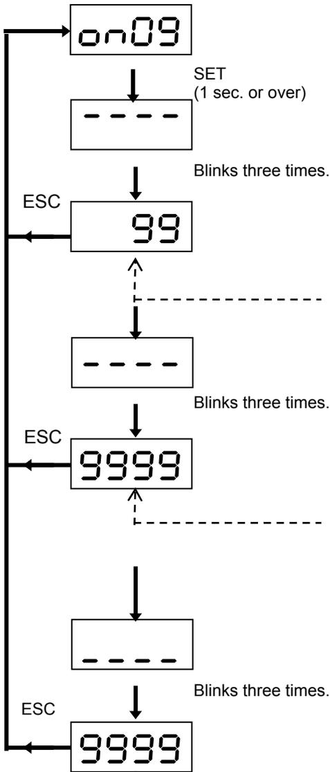
The difference between the command position and feedback position is displayed. The unit of deviation amount follows the deviation unit selected in PA1\_31.
