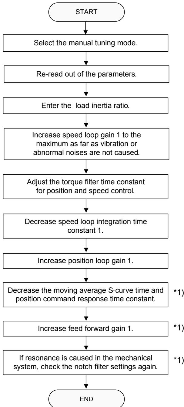
\*1) Adjustment is unnecessary under speed control.
