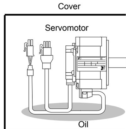
To install the servomotor vertically or at an oblique direction, route the cables to secure a cable trap (see the figure on the right).
