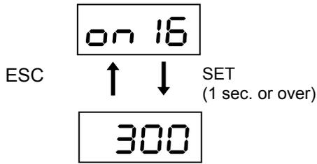
The DC link voltage (min.) of the servo amplifier at every two seconds is displayed.
