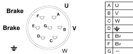
Brake connector kit (Motor side)
