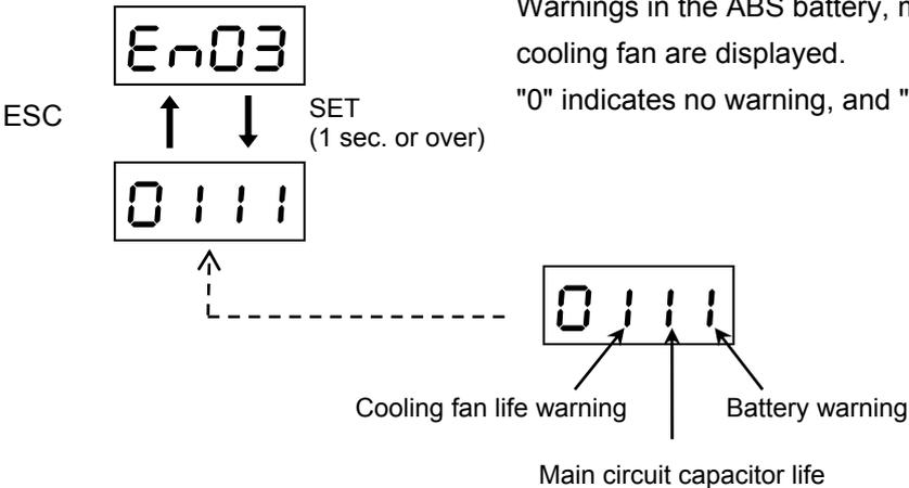
Warnings in the ABS battery, main circuit capacitors and cooling fan are displayed.
