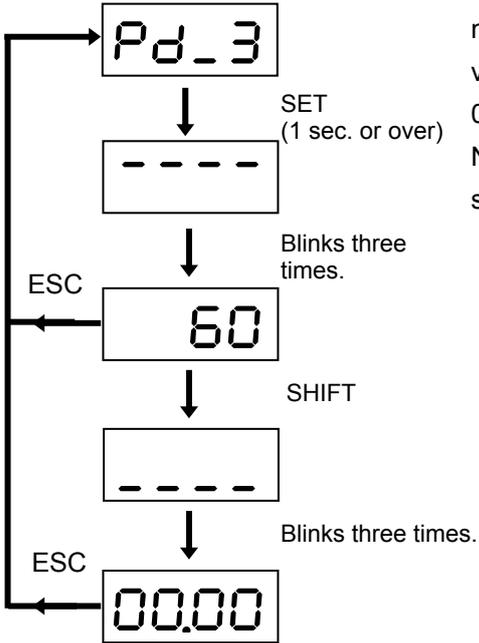
Set the travel speed to the motor target position. Use the motor shaft rotation speed for the setting value. The setting value range is from 0.01 to 6000.00 r/min in increments of 0.01. Note that the setting speed is not the machine travel speed.
