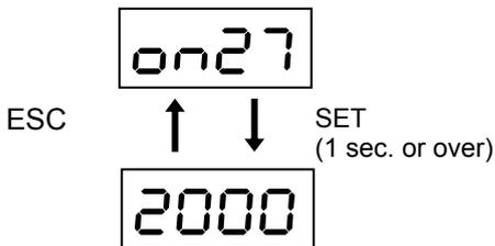
The resonance frequency recognized by the servo amplifier is displayed.
