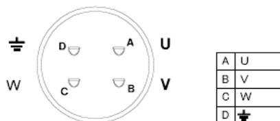
Motor power connector kit (Motor side : With brake)
