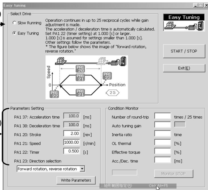
**Hint** Slow running is unnecessary for machines with a rotary driving system.
