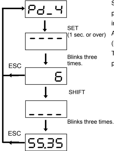
Set the stop time after the motor has reached the target position. The setting value range is from 0.00 to 655.35 s in increments of 0.01. After the stop time has elapsed, the sequence output signal (in-position signal [INP]) turns on. The decimal point position can be changed in the parameter PA2-42 (timer data decimal point position).
