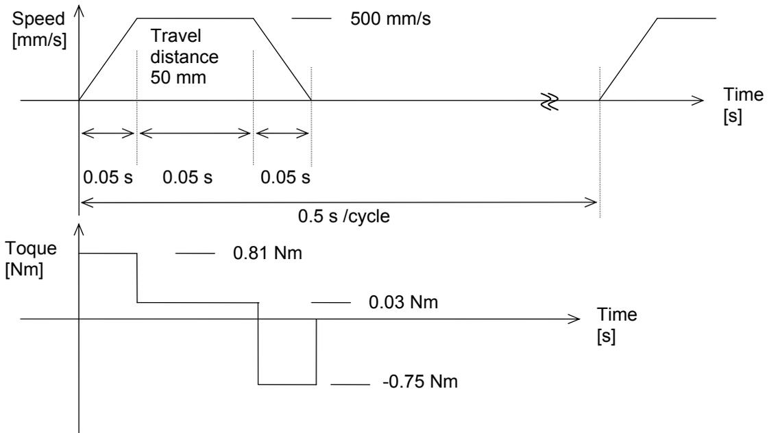
This profile is based on calculation selection. The operation cycle time supposes 0.5 s.
