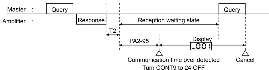
If PA2\_95 is set to 0.00 s, communication time over is not detected. Use this setting as needed, for example, if the system communicates periodically and you wish to detect discontinuation of the communications.
