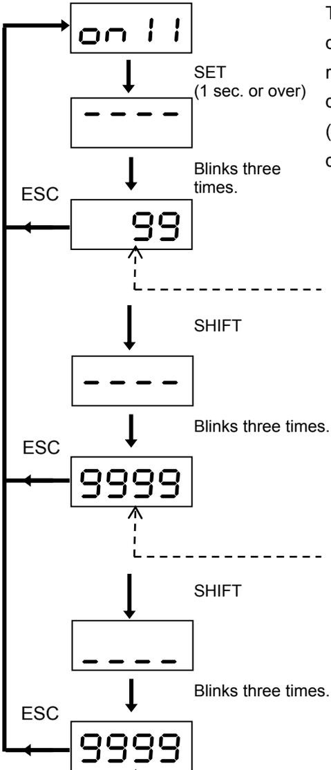
The cumulative pulses of servomotor rotation amount are displayed in encoder pulses (1048576 pulses per revolution with 20-bit serial encoder). Reverse rotation decreases the cumulative value. Even if the load (mechanical system) rotates the motor, the correct value is displayed.
