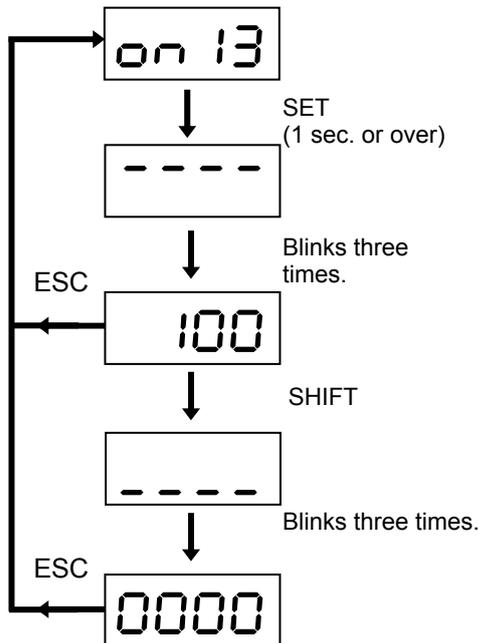
The number of pulses in a homing counted since the home position LS signal is turned off until the Z-phase of the encoder of the servomotor is detected is displayed. The indication is updated every time homing is performed. Because the value is in the homing direction, no negative sign is attached.
