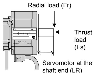
Radial load: the load applied vertically to the motor shaft
