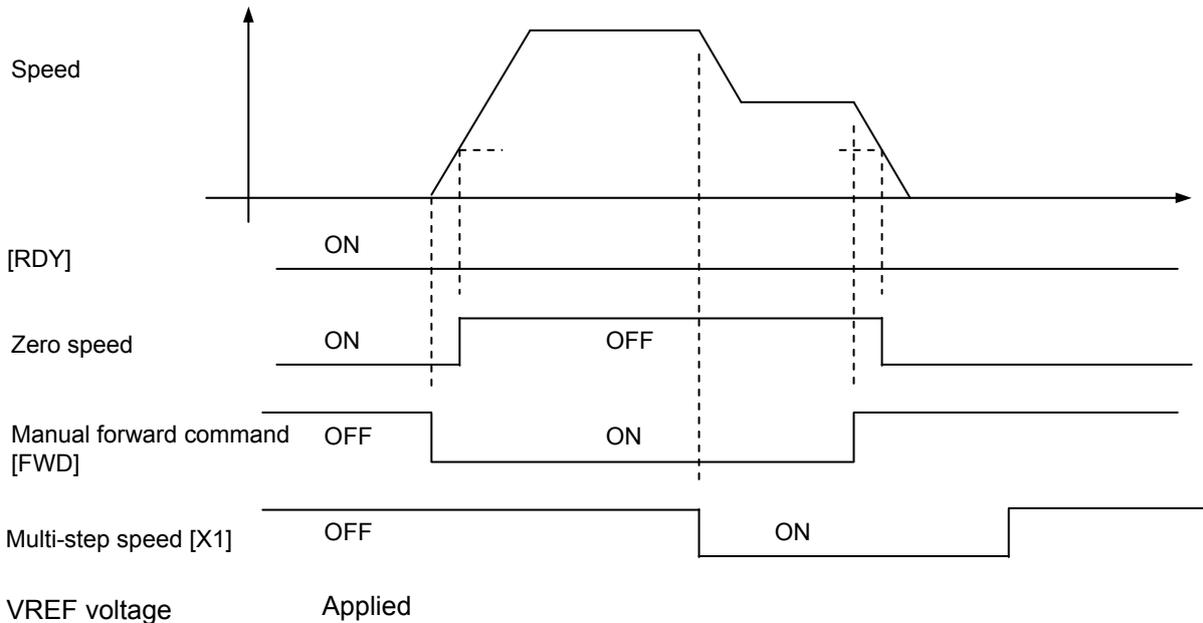
Use parameter PA3\_35 to specify the zero clamp level in relation to the [VREF] input.
