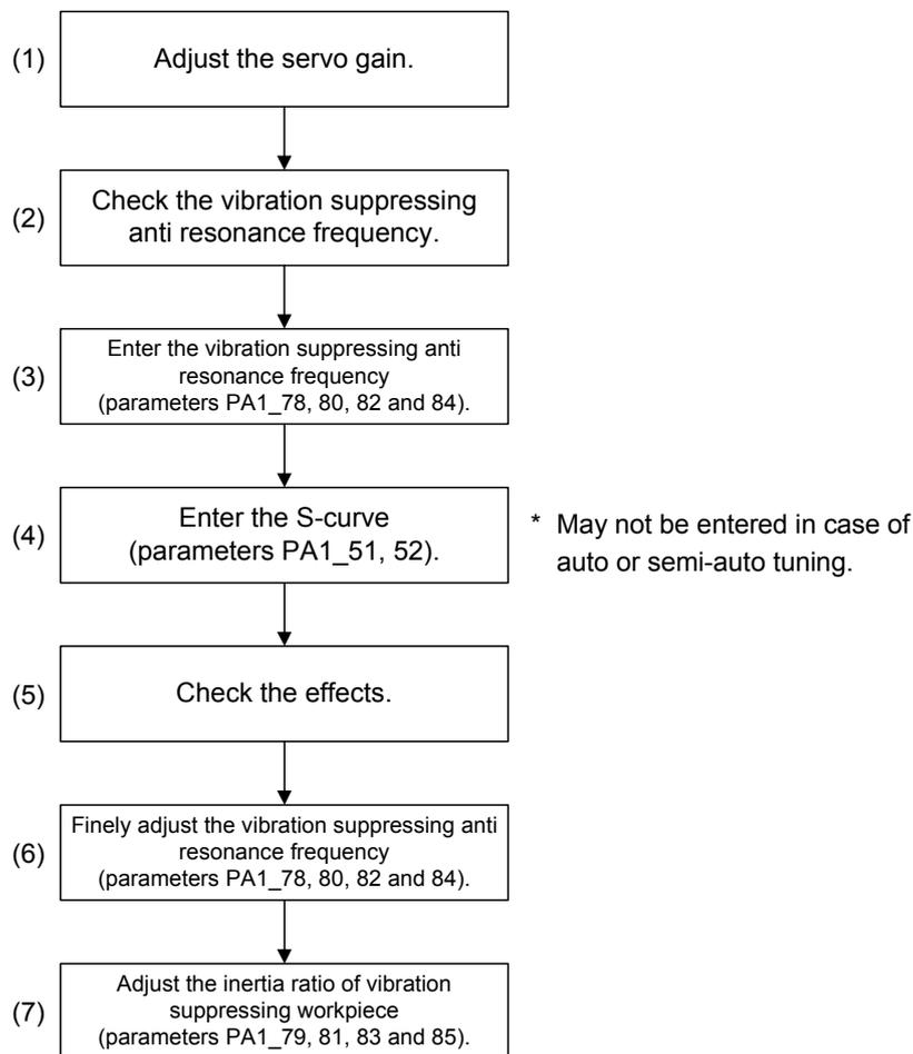
(1) Adjusting the servo gain
