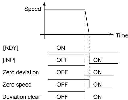
**Note** The in-position [INP] signal shown in the figure indicates the state in the level output mode.
