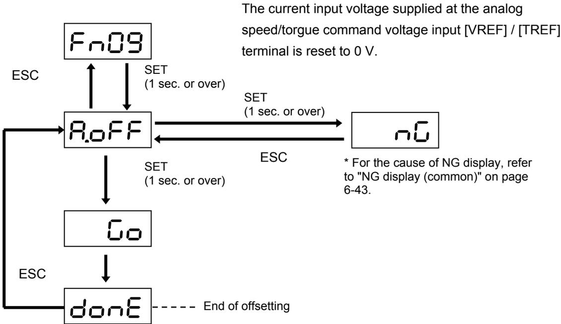
If both the X1 and X2 terminals of multi-step speed selection are turned off with the FWD (REV) signal, the output shaft of the servomotor rotates according to the analog speed command voltage. The output shaft of the servomotor may rotate at a small speed even if the speed command voltage is 0 V.
