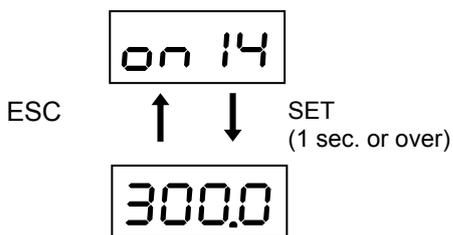
The load inertia ratio recognized by the servo amplifier without relations to parameter PA1\_13 (tuning mode selection) is displayed. The value is displayed in a multiple (in 0.1 increments) to the inertia of the servomotor itself. The displaying range is from 0.0 to 300.0 times.
