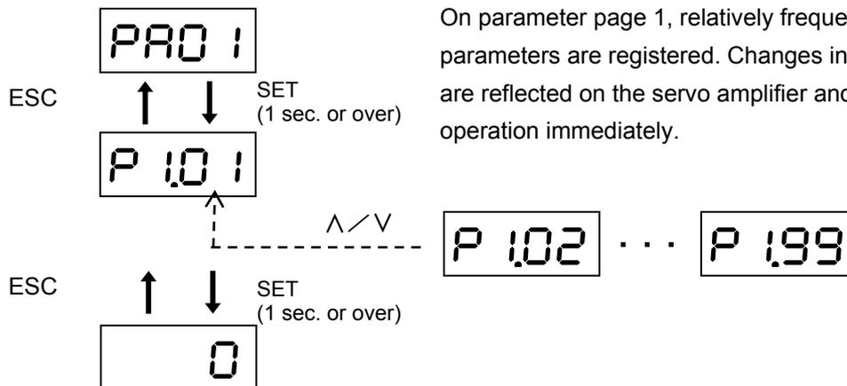
On parameter page 1, relatively frequently used parameters are registered. Changes in most parameters are reflected on the servo amplifier and servomotor operation immediately.
