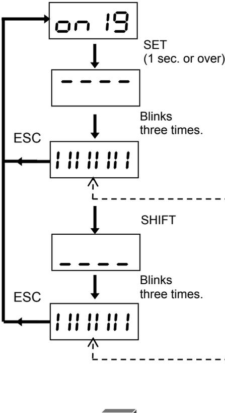
The ON/OFF status of sequence input signals supplied to the servo amplifier is displayed.
