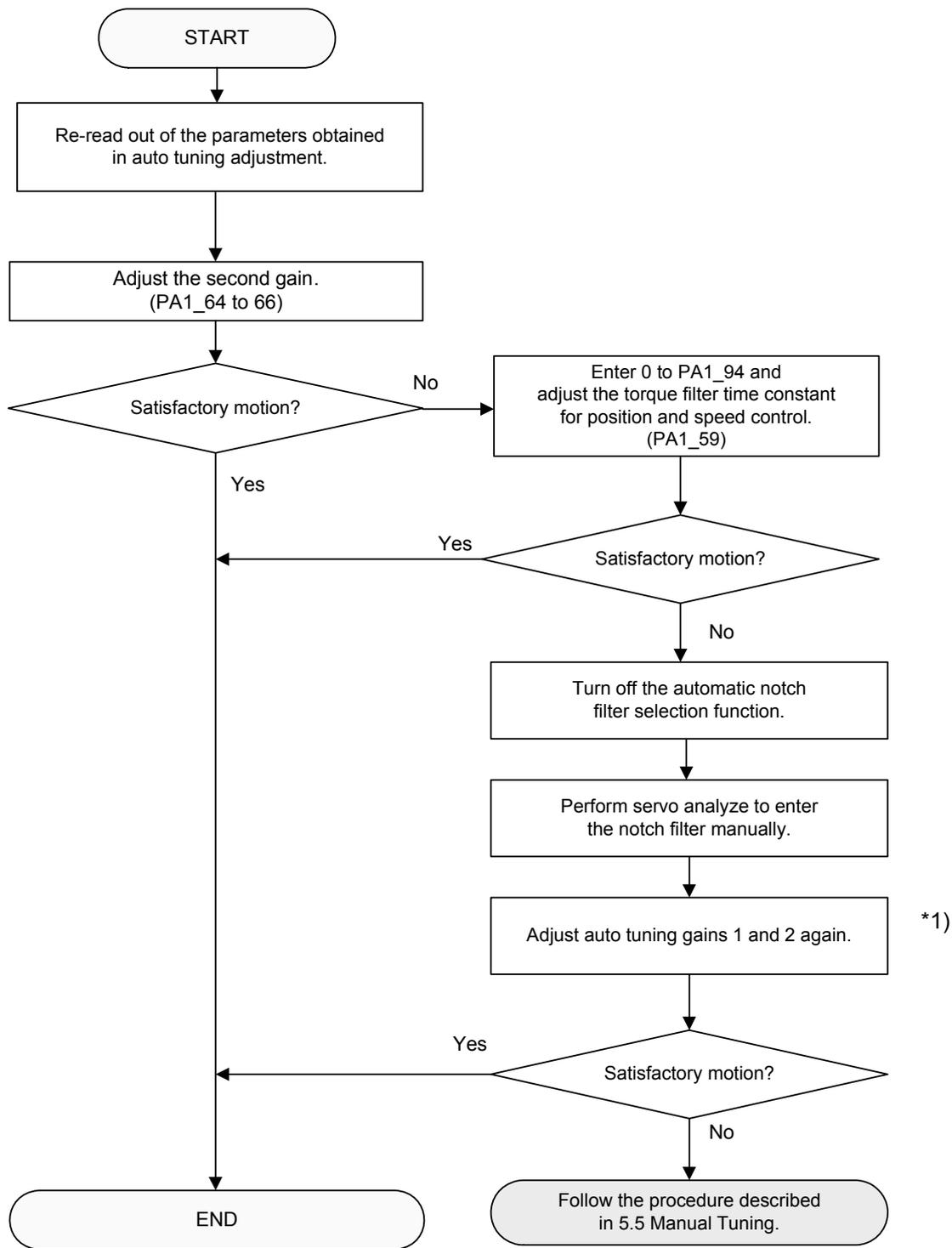
\*1) Adjustment of auto tuning gain 2 is unnecessary under speed control.
