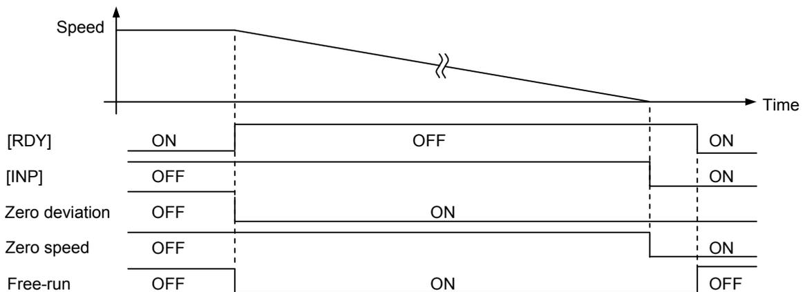
**Note** In regular cases, free-run is not used for vertical traveling machines. If the function is used for a vertical traveling machine, examine adaptability with the brake carefully.
