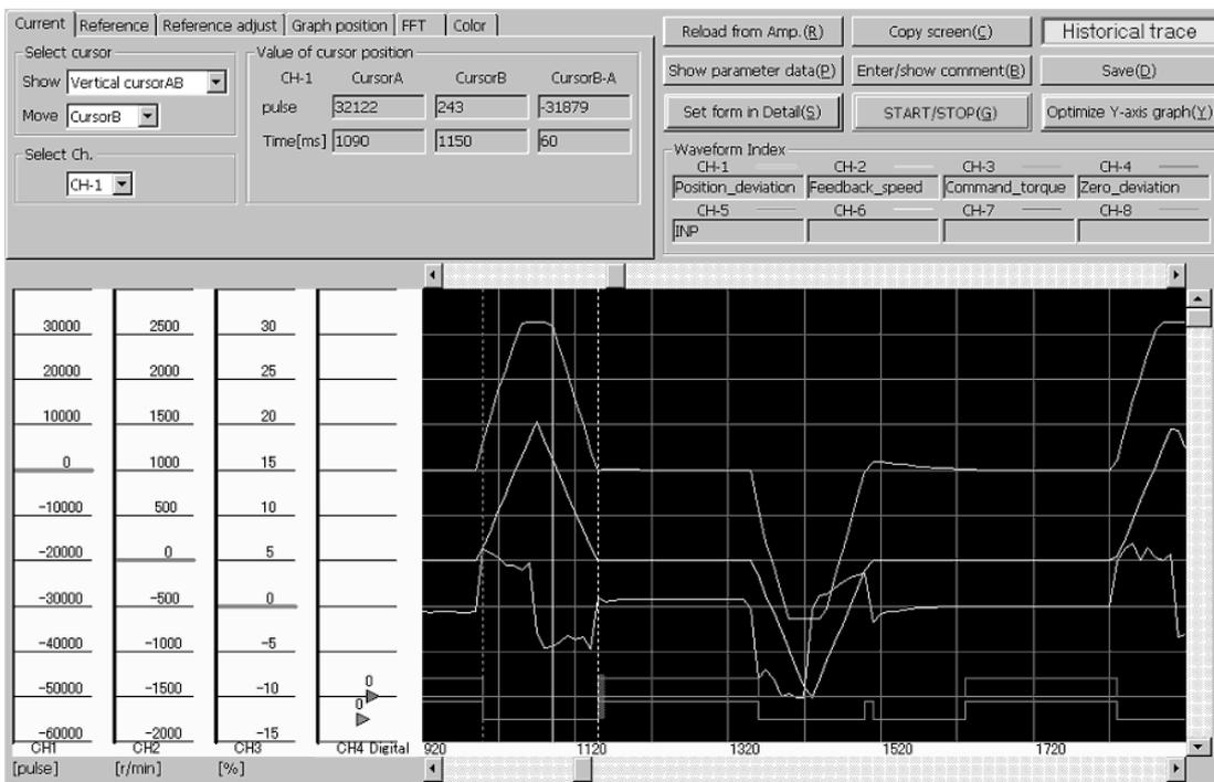
You can show the interval between two points, overlap waveforms, perform FFT analysis, re-load the waveform, copy the screen, show parameter data of the acquired waveform, save the waveform (in a CSV file), or do other things.
