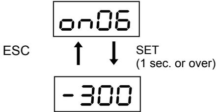
The load ratio of the servomotor; displayed in percent to the rated torque.
