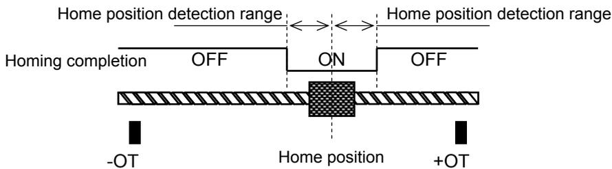
The zero position is not necessarily 0. The home position is the position specified as a home position after homing completion (PA2\_16) or preset position (PA2\_19).
