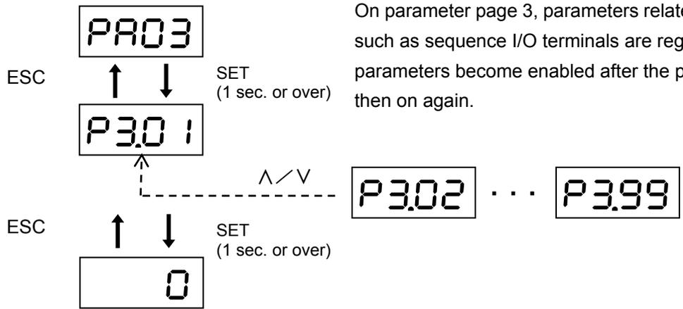
On parameter page 3, parameters related to system setting such as sequence I/O terminals are registered. Changes in parameters become enabled after the power is turned off then on again.
