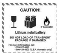
Fig.1 Label to be attached to the package outer surface
