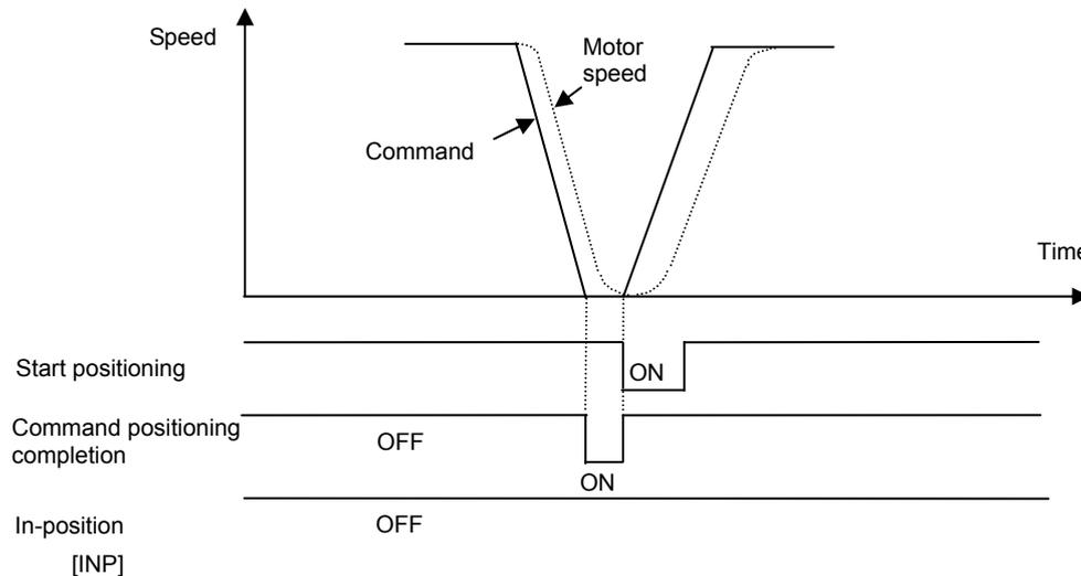
If a motion to the current position is started, the servomotor does not start but the in-position signal is turned off for the time specified in PA1\_34 (in-position minimum OFF time / single shot ON time).
