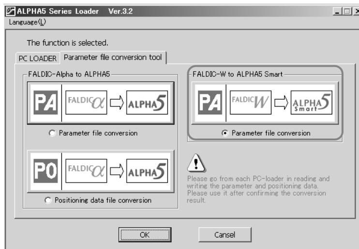
How to convert the file from the parameter file for FALDIC-W series to the one for ALPHA5 Smart series is explained on the next page.
