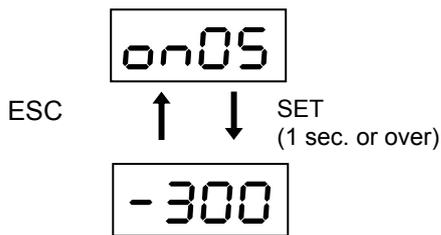
Peak torque value of the servomotor at every two seconds; the torque is displayed in percent to the rated torque. The range from 0% to the maximum torque is displayed in increments of 1. In case of a negative peak torque, a negative sign is attached to the most significant digit.
