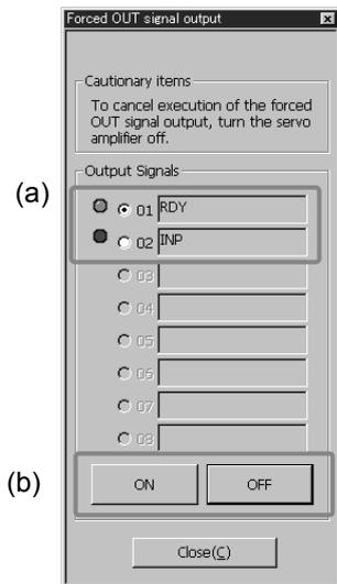
Select the OUT signal output at (a) and select ON or OFF at (b).
