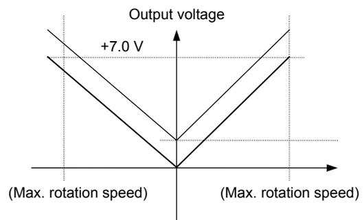
Specify the negative sign for the monitor 1/2 scale to reverse the polarity of the output voltage.
