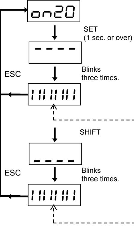
The ON/OFF status of sequence output signals issued by the servo amplifier is displayed.
