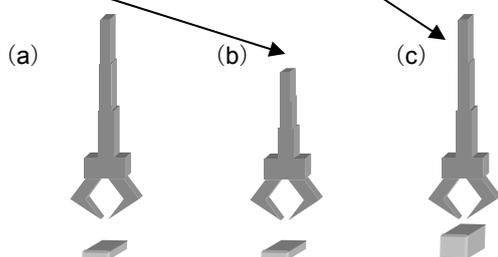
The vibration suppressing anti resonance frequency varies according to conditions a, b and c.
