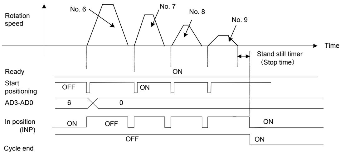
• Positioning data are regarded as being executed while timer is measured.
