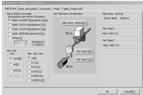
Enter the specifications of the machine to automatically calculate the settings. Parameters grouped according to each mechanical configuration helps you enter simply.
