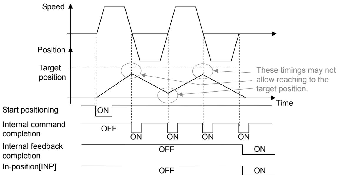
Setting value: 1 (Internal feedback completion.)
