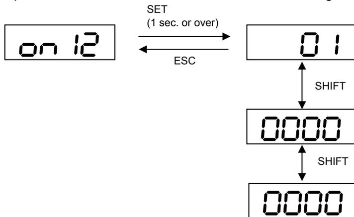
The display example for 10000000-pulse is shown.
