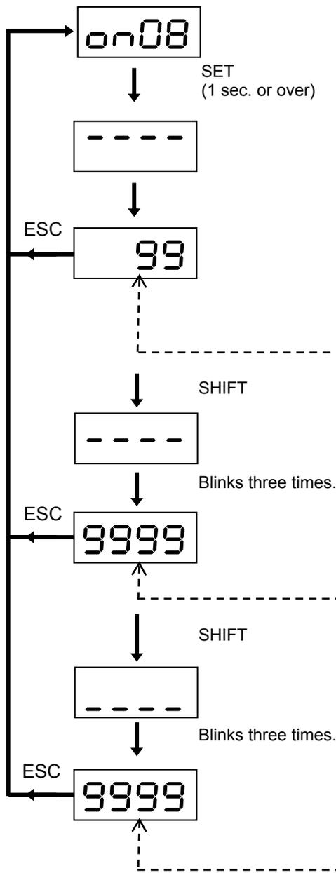
The position of the servomotor controlled by the servo amplifier is displayed in the unit amount after correction with an electronic gear. If the operation command is turned off and the load (mechanical system) rotates the motor after the target position is reached, the position is not correct.
