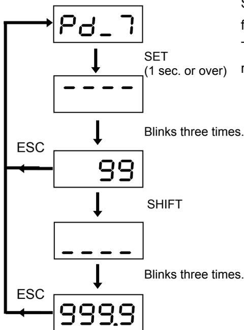
Set the motor deceleration time. The setting value range is from 0.0 to 99999.9 ms in increments of 0.1. The setting value is the time until the motor rotation speed reaches 2000 r/min.
