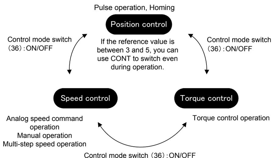
[Example] The operation pattern of control mode selection 3 (position ↔ speed) is shown in the figure below.
