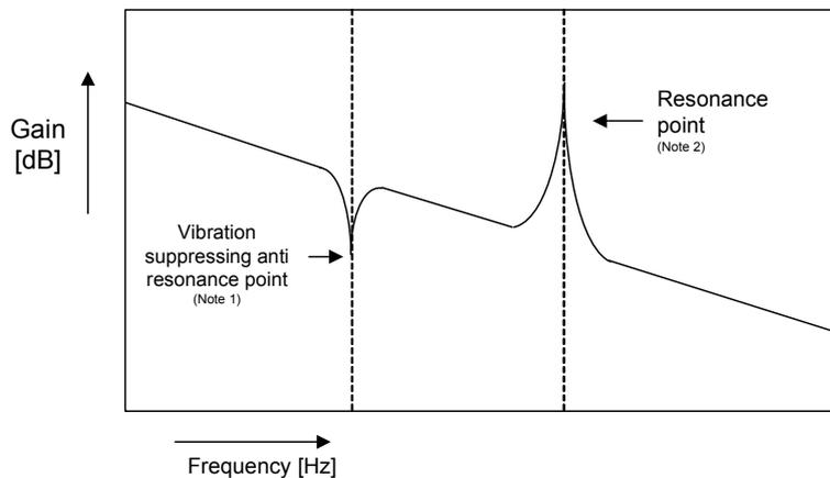
Note 1 The vibration suppressing anti resonance point may not be observed with the servo analyze function in the following machine configuration.
