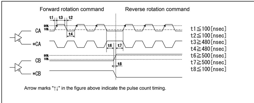
■ Open collector input, command pulse/direction (reference value of parameter 03: 10)
