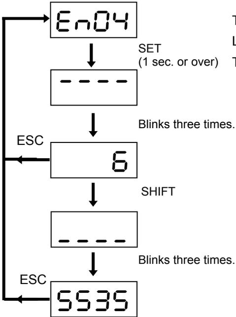
The cumulative time of turning the main power (L1, L2 and L3) on is displayed.
