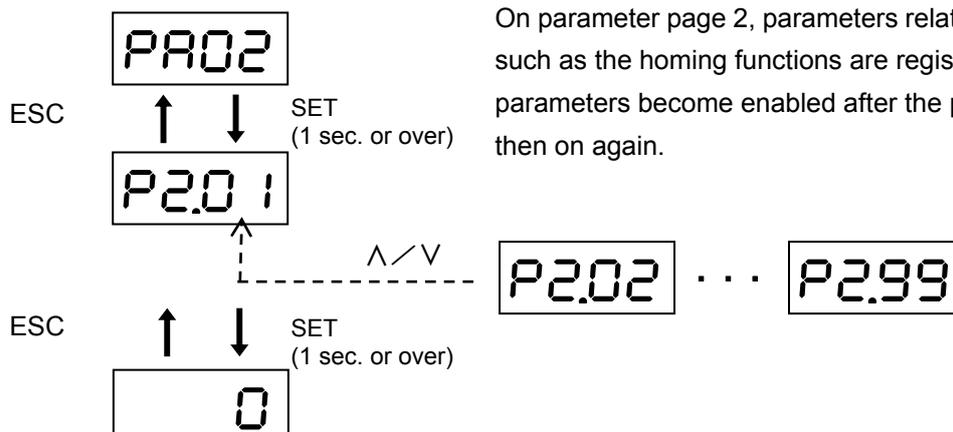
On parameter page 2, parameters related to system setting such as the homing functions are registered. Changes in parameters become enabled after the power is turned off then on again.
