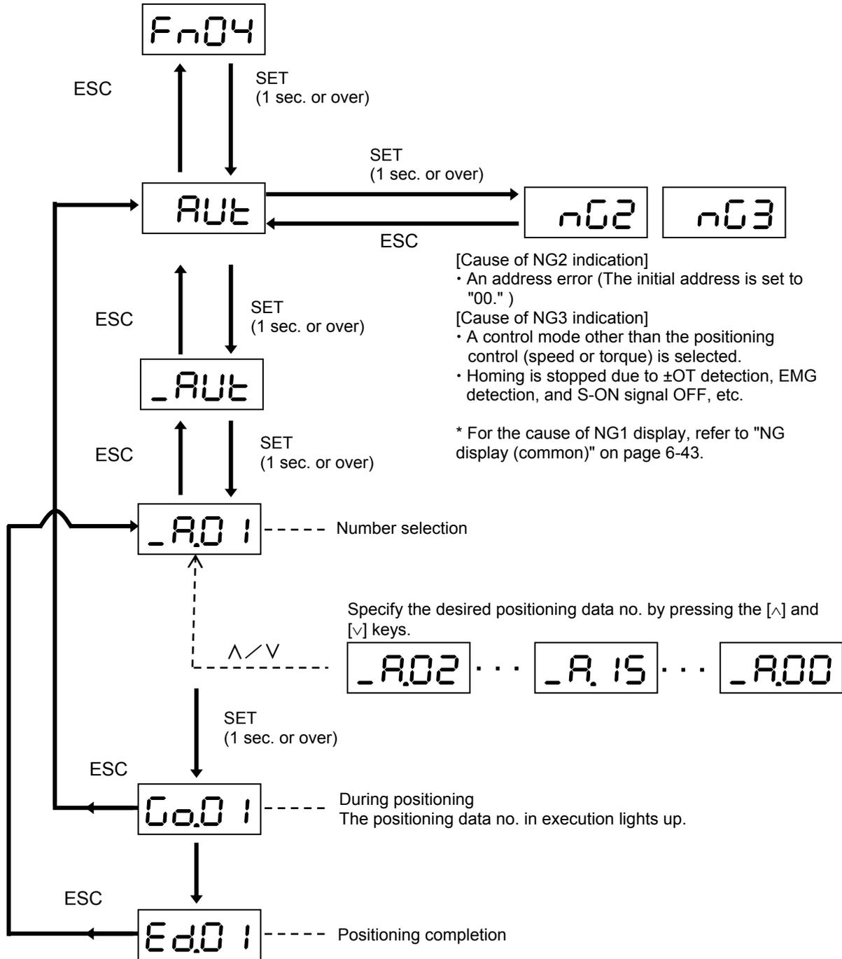
**Note** The forced stop, external regenerative resistor overheat,  $\pm$ OT and free-run signals are enabled even during test operation. Check these signals if test operation does not start.
