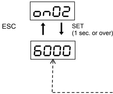
Current speed command issued to the servomotor. The command speed is given in a speed command voltage, multi-step speed, pulse or similar. The speed is displayed in r/min and a negative sign is attached for reverse rotation (clockwise rotation when viewed against the motor shaft).
