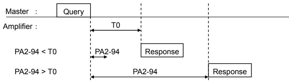
After the master has sent a query, if it takes a long time until the master switches into the receiving state, set PA2\_94 (response time) as needed because responses from the amplifiers might not be received correctly.
