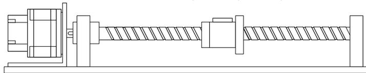
$$\frac{\text{(Traveling amount of mechanical system per servomotor revolution)}}{1048576 \text{ pulses/rev}} \times \frac{\text{Numerator 0 of electronic gear}}{\text{Denominator of electronic gear}} = \text{(Unit amount)}$$
