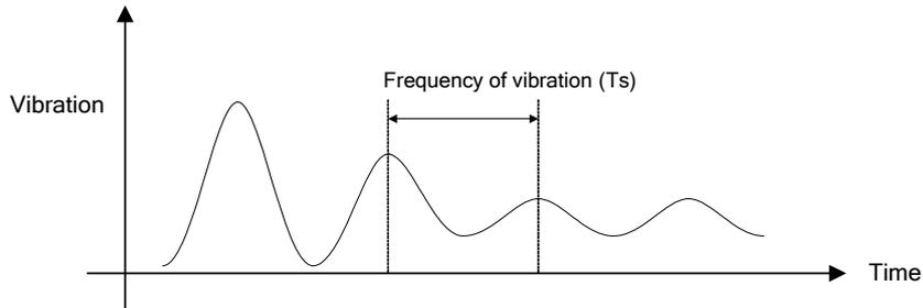
$$\text{Vibration suppressing anti resonance frequency} = \frac{1}{T_s} \text{ [Hz]}$$
