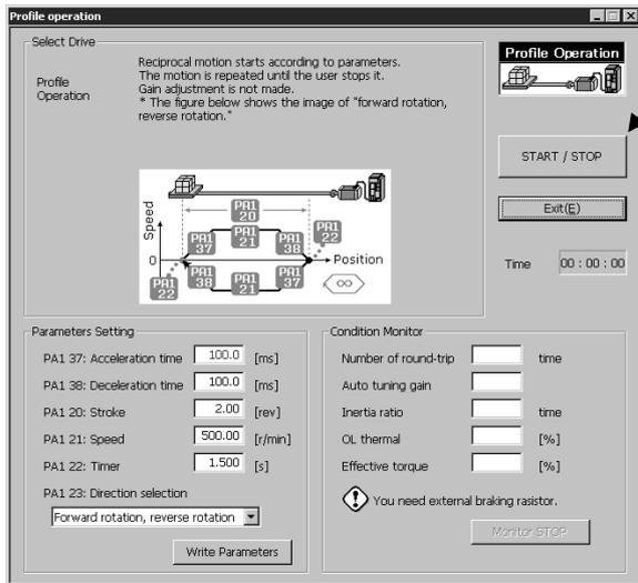
Press the "START/STOP" button to start profile operation.
