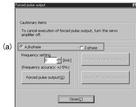
Select the pulse signal to be output, at (a).
