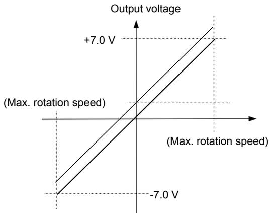
Monitor 1 terminal (output on single polarity)
