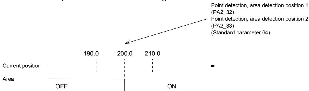
(3) Area ON → OFF (If PA2\_31 (point detection, area detection) is 2)
