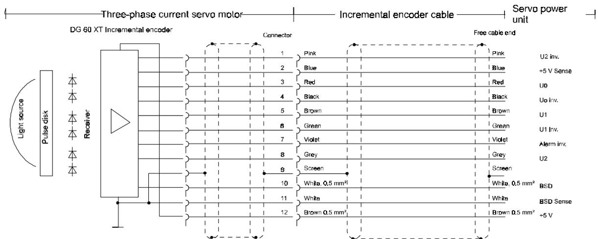
Two different versions of the cable are supplied that are pre-cut and have integrated Interconnectron PLD 121 circular plugs. You must only use original manufacturer parts that guarantee contact protection, tension relief, protection levels and permanent contact.
