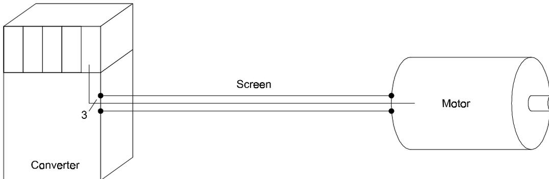
Connecting the screen to frame ground at both ends ensures that the conductor does not leave the screening "system housing".
