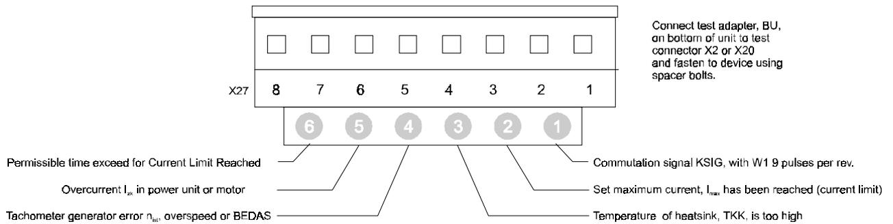
• Fault Evaluation BUS 3 Servo Power Unit
