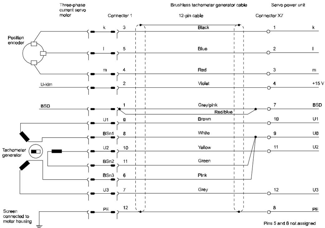
Connect the sub-unit terminal to socket X7 on the controller. If necessary, unscrew the sub-unit terminal before laying the cable.
