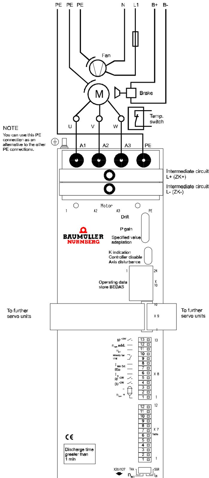
5.3.4 Double-Axis BUS 20 Connection Diagram
