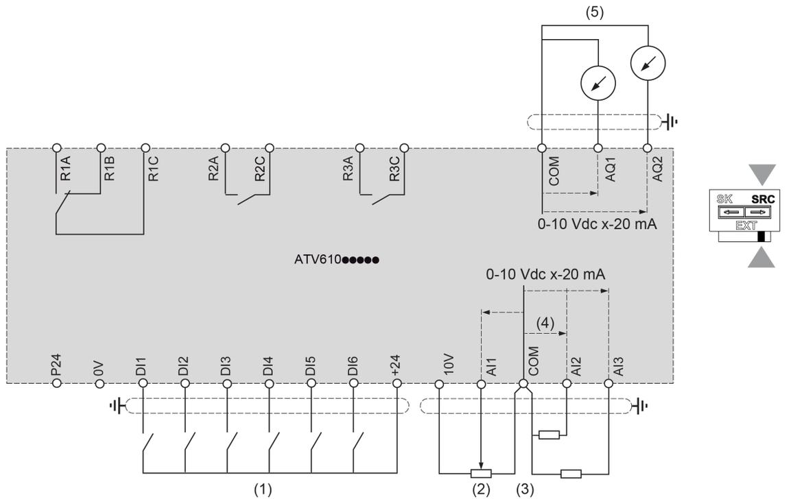
(1) Digital Inputs - Shielding instructions are given in the Electromagnetic Compatibility section, page 89.
