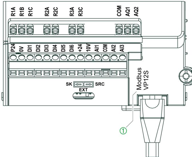
① Modbus VP12S: This is the standard Modbus serial link marking. VP•S means connector with power supply, where 12 stands for the 12 Vdc supply voltage.
