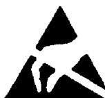
**Modules contain electrostatically sensitive components**
